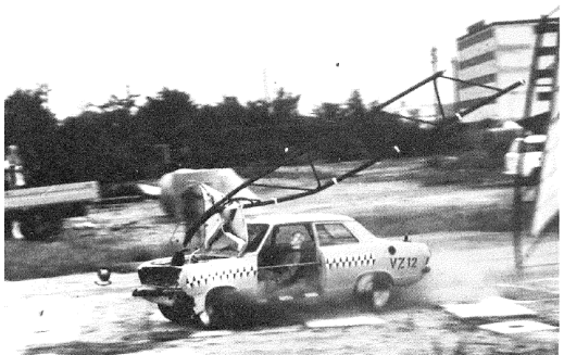
Figure 5.15: Vehicle and structure impact behaviour. Left: real impact test [45]. Right: numerical impact test.
