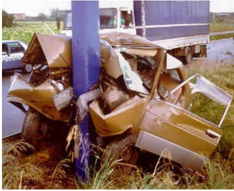
Figure 1.1: Consequences of a vehicle colliding into various types of columns. Left: rigid column. Right: deformable column.
